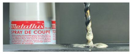
**Description:** Universal cutting foam for any metal, from the hardest stainless steel and titanium to soft metals like copper, brass, aluminum and cast metal. Can be universally used for all cutting and working processes.
